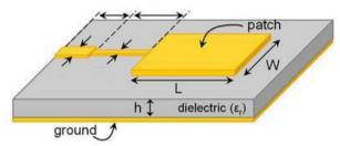
Fig. 1.2.Structure of a patch antenna.
